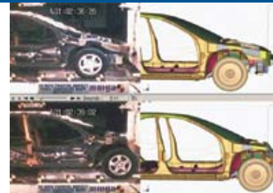
Excellent correlation between the simulated and actual full vehicle crash events is achieved through extensive component /subsystem testing and meticulous model definition.
