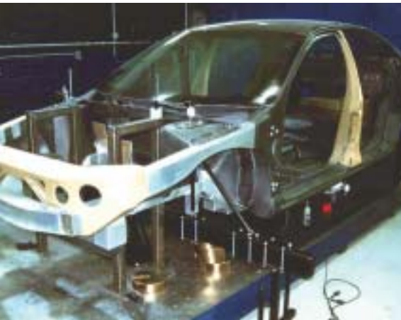
Large surface plates support a wide range of test classes and magnitudes. Purpose built fixturing assures accurate and consistent results.
