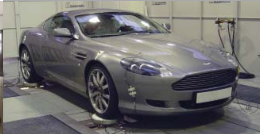
With in-house designed and built multi-post rigs in Europe and North America, Multimatic can service the global automotive OEM and racing communities.
